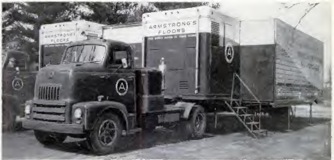
By parking two big trucks, each with expanding walls, alongside each other and coupling them as shown below, this company hauls its own mobile auditorium seating 100 persons anywhere in the country for sales meetings
